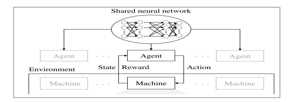
2. State, action, and reward are proposed to address the variabilities in production requirements and initial setup status
